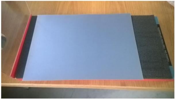
Open the Lid of the cutting die and position your sample on the foam base.
