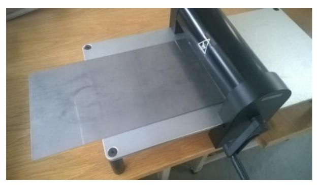
Place the metal tray onto the bed of the universal cutter.
