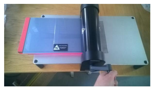
Once the cutting die has entered the rollers rotate the handle.
