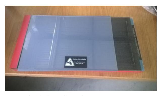
Close the Lid and check the alignment of your sample. Maximum sample width is the width of the cutting die.
