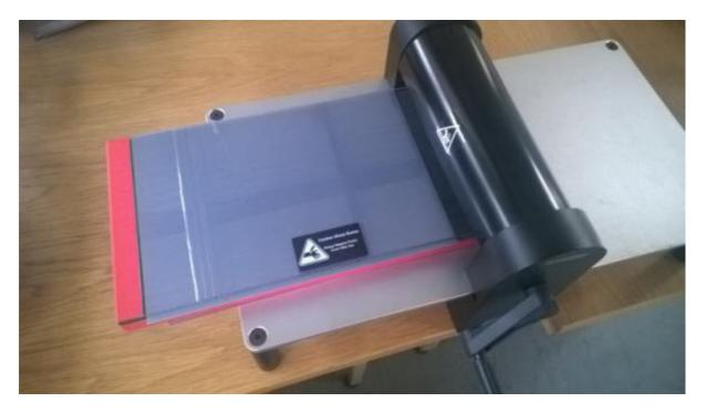
Place the cutting die on top of the metal tray with the open end of the die towards the roller. Push the cutting die into the rollers.
