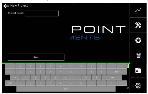
Enter the project name using the onscreen keyboard and press save. The instrument will now enter the open project menu.
