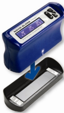
Place the instrument in the calibration holder.
