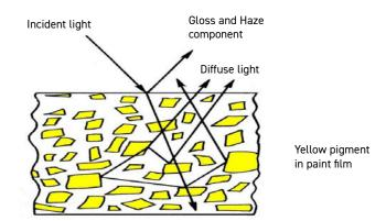
The Novo-Gloss compensates for reflection from within the coating for highly reflective pigments, metallic coatings and speciality pigments, allowing the haze of any painted surface to be measured.
