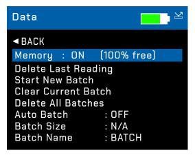
The Data & Batch Screen is similar in functionality to that of the menu screen but also allows the selection and setting of the Auto Batch size.
