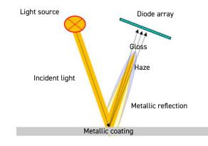
The Novo-Gloss captures compensation information from a region adjacent to the haze measurement angle, this means it can be used on metallic coatings which reflect light directionally
