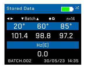
When Memory is set to ON (as detailed later in the Menu Screen section of this manual) measurements can be recalled and displayed from any batch stored in the Novo-Gloss memory.
