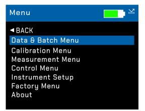
The Setup Screen is used to customise the instrument to the user's preference. Press the Up / Down buttons to navigate through the options, press the Enter button to select the option required.
